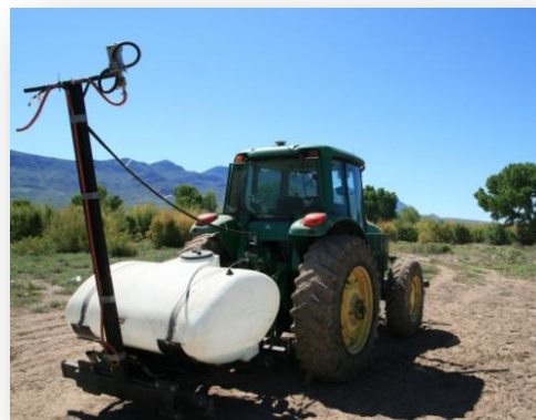
Application equipment: Left photo is a custom made carpet roller; right photo is the sprayer used to treat salt cedar where the nozzles emit a spray stream reducing potential for off target movement of herbicide.
